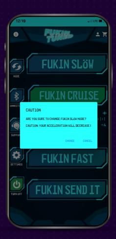
Fukin Slöw: Select the Fukin Slöw Mode and choose 'Change'. This mode deliberately reduces the throttle response to enhance control in challenging weather and land conditions.
